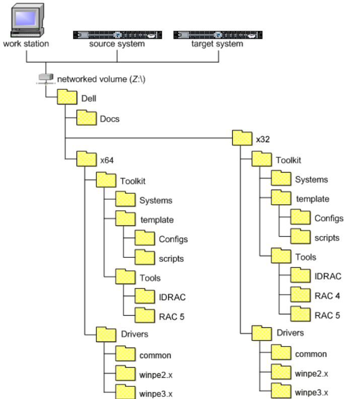
Figure 3-1. Sample DTK Default File Structure
